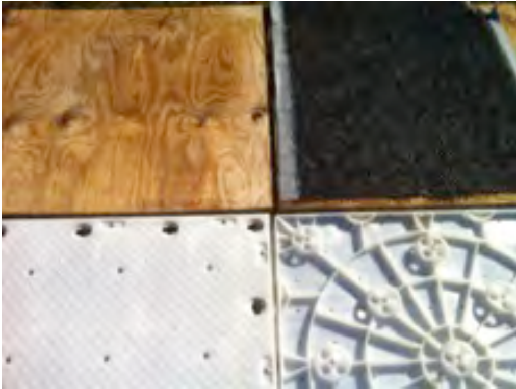
Figure 3. Treatments included Plywood (top left), Plywood + Enkamat (top right), Matrax (bottom left), and Terratile (bottom right). Photo: John Royse
