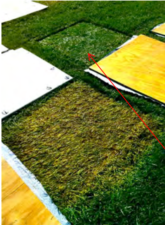
Figure 13. Effects of three cover types on turf and soil impacts. Left: Matrax (Top) and Plywood + Enka (bottom) caused matting over of the shoots. Right: Terratile sunk into turf/soil (when driven over) resulting in turf damage (beginning of the 2010 fall trial).
